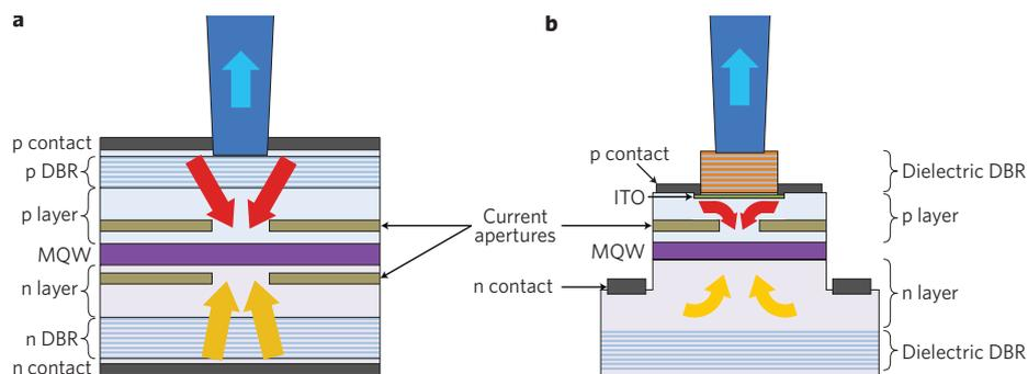
**Figure 1** | VCSEL designs. **a**, Standard VCSEL. **b**, Nitride blue-green VCSEL using a pair of dielectric DBR mirrors and intracavity contacts on the p-layer side to enhance hole injection into the centre of the cavity region. Red, hole injection; yellow, electron injection; and blue, laser emission.
